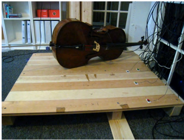
FIGURE 3. View of the tested stage floor prototype, showing the 4 accelerometers tightly mounted to the wood surface using strong double-sided adhesive tape.
