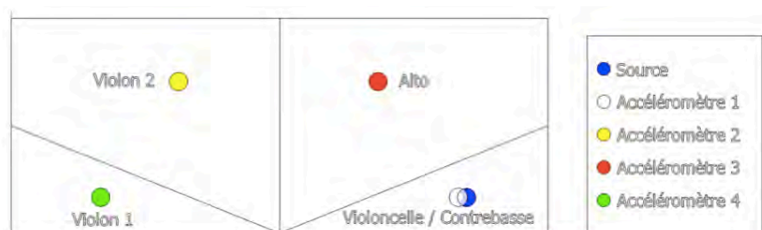
FIGURE 5A. Schematic plan showing the location of the vibration source (cello and tapping machine) and the 4 accelerometers for the on-stage measurements.
